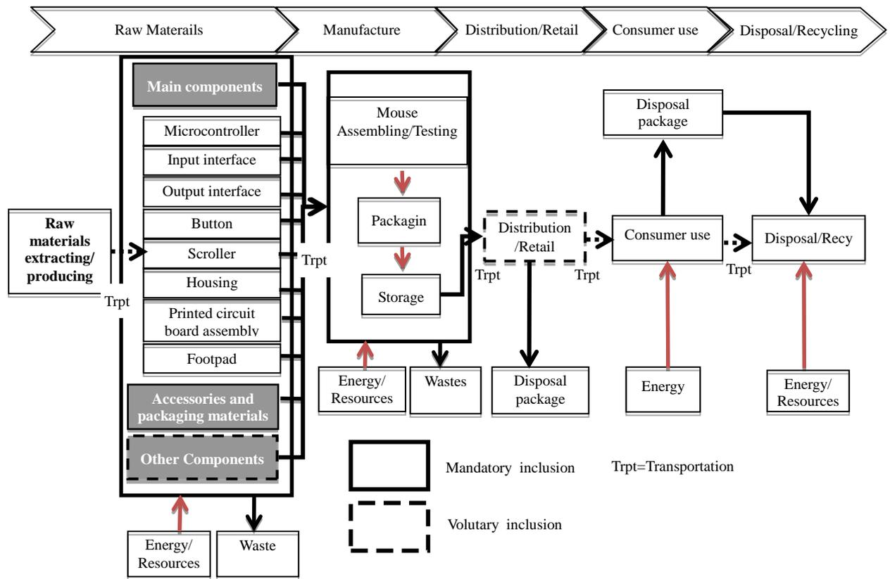
Figure 1 System boundary of the main product system
